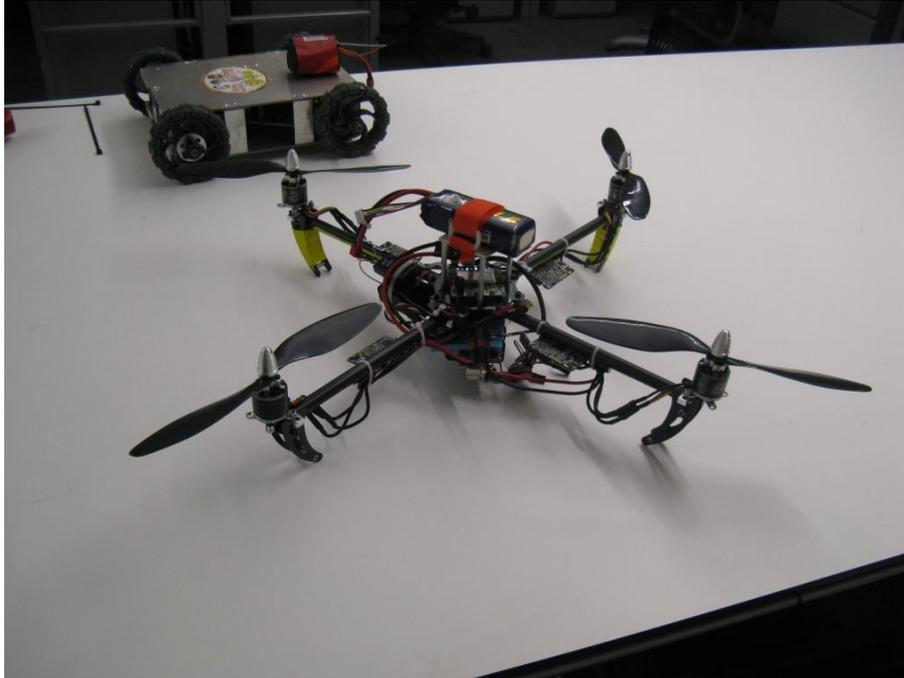
**Figure 49:** Four FFv1.2s boards on a multirotor with 10” propellers.
