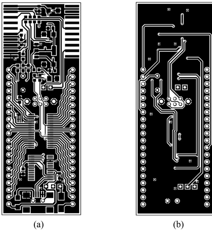
**Figure 6: The Wootstick circuit board copper patterns for the top (a) and bottom (b) layers. All components are located on the top layer for ease of assembly.**
