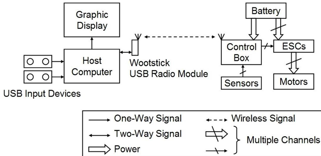
**Figure 2: The system configured to drive high-power motors with external electronic speed controllers (ESCs). The control box sends signals to the speed controllers, which then channel power to the motors.**
