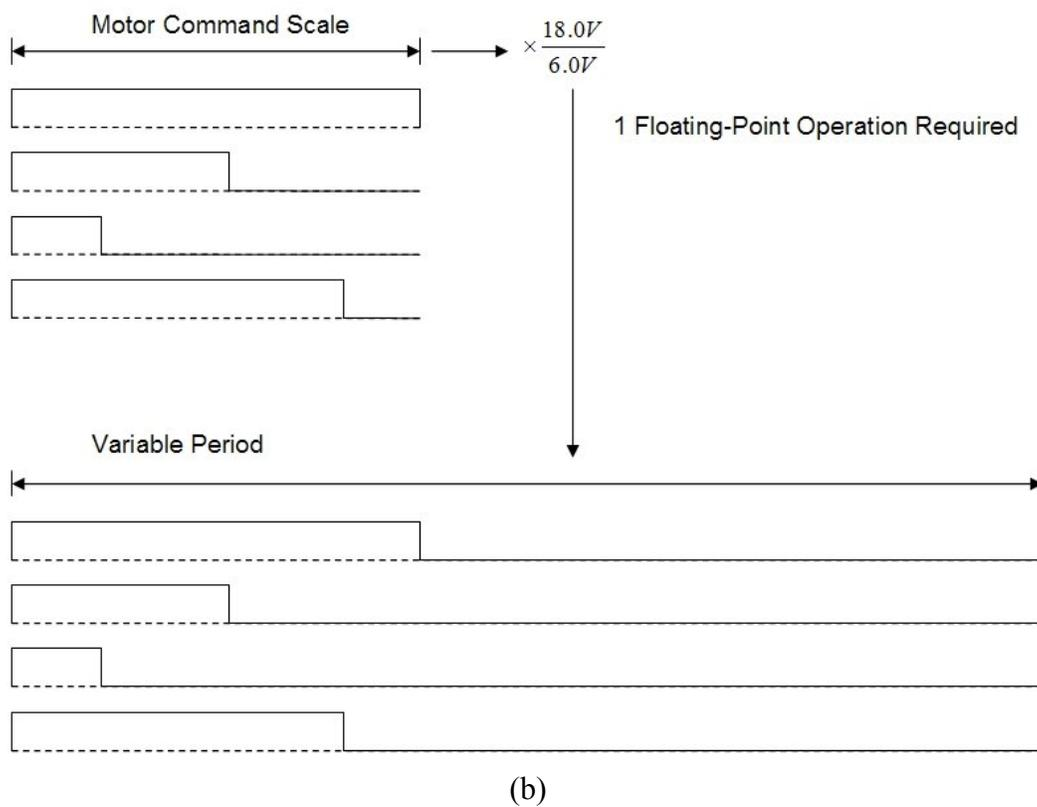
**Figure 11: The method of scaling motor commands to account for battery voltages above the highest rated motor voltage. Fixed-frequency operation (a) has been replaced by variable-frequency operation (b) to minimize the computation required.**
